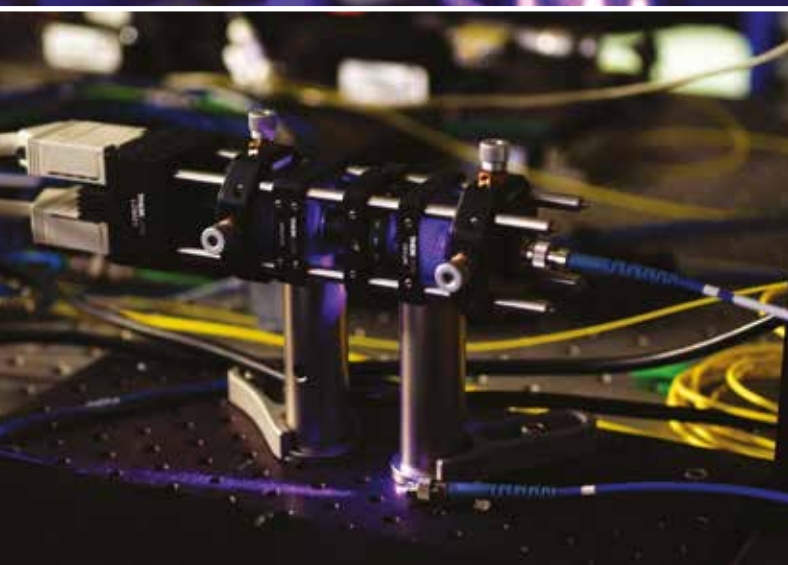
Component of the NQIT entangler that couples the light emitted from ion traps into an optical fibre for testing the loss and extinction of fibre components / Paul Gow & Paola Mennea
