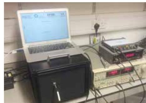
*Magnetometer being developed by the University of Warwick, using nitrogen-vacancy centres in diamond / Gavin Morley*
