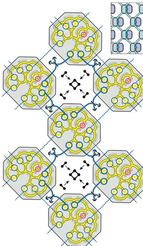
Schematic showing advanced ion trap chips, each a 2D grid of pathways along which atoms travel, networked together to form a computer / *Simon Benjamin*
