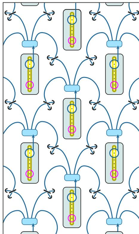
Schematic showing how simple ion trap chips, devices with a few trapped atoms within, can be networked to form a computer / *Simon Benjamin*
