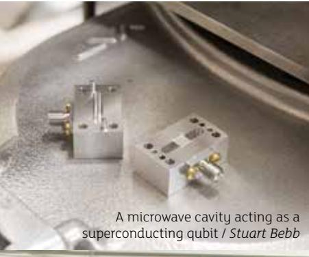
A microwave cavity acting as a superconducting qubit / Stuart Bebb
