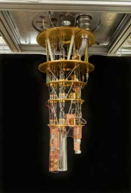
Customised dilution refrigerator for operation of quantum microwave circuits at less than a degree above absolute zero / Stuart Bebb
