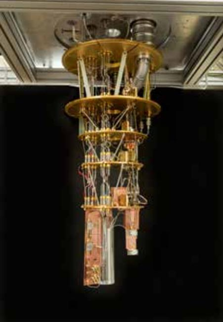
Customised dilution refrigerator for operation of quantum microwave circuits at less than a degree above absolute zero / Stuart Bebb
