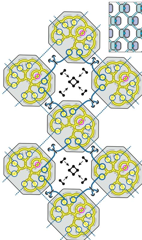
Schematic showing advanced ion trap chips, each a 2D grid of pathways along which atoms travel, networked together to form a computer / *Simon Benjamin*
