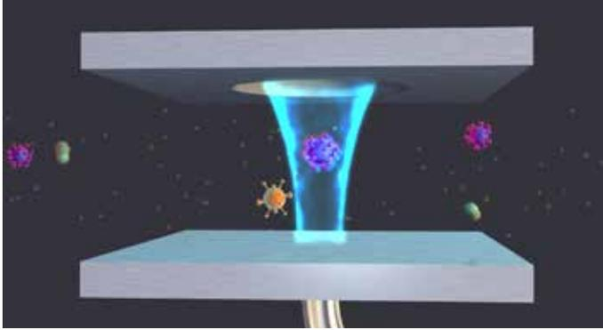
Schematic showing a microcavity being used as a sensor for biological pathogens / Photonic Nanomaterials Group, University of Oxford
