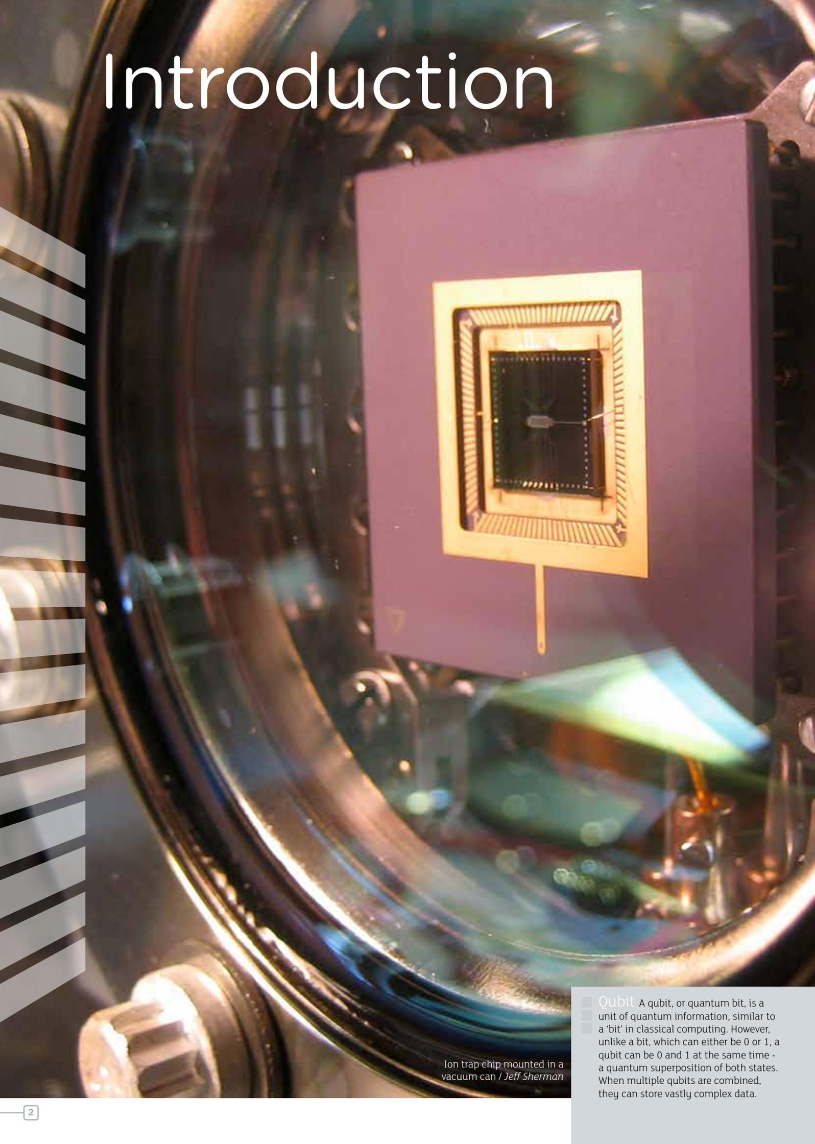
Ion trap chip mounted in a vacuum can / Jeff Sherman
