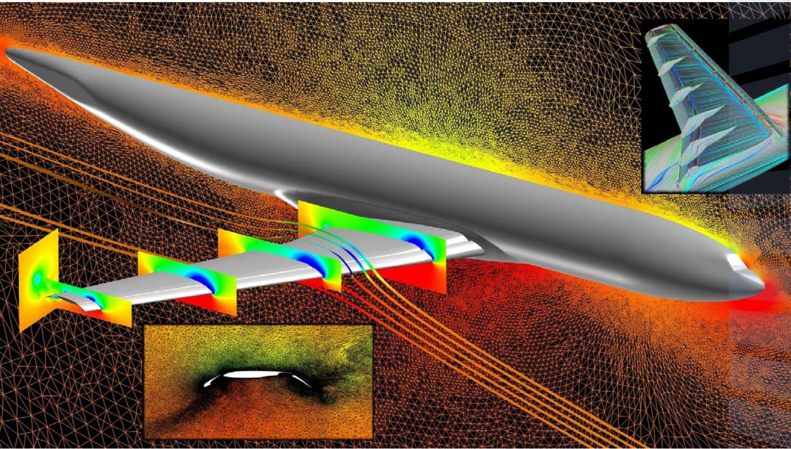
A computational fluid dynamics (CFD) visualization produced using a NASA supercomputer, showing a mesh adaptation used to simulate a transport aircraft
