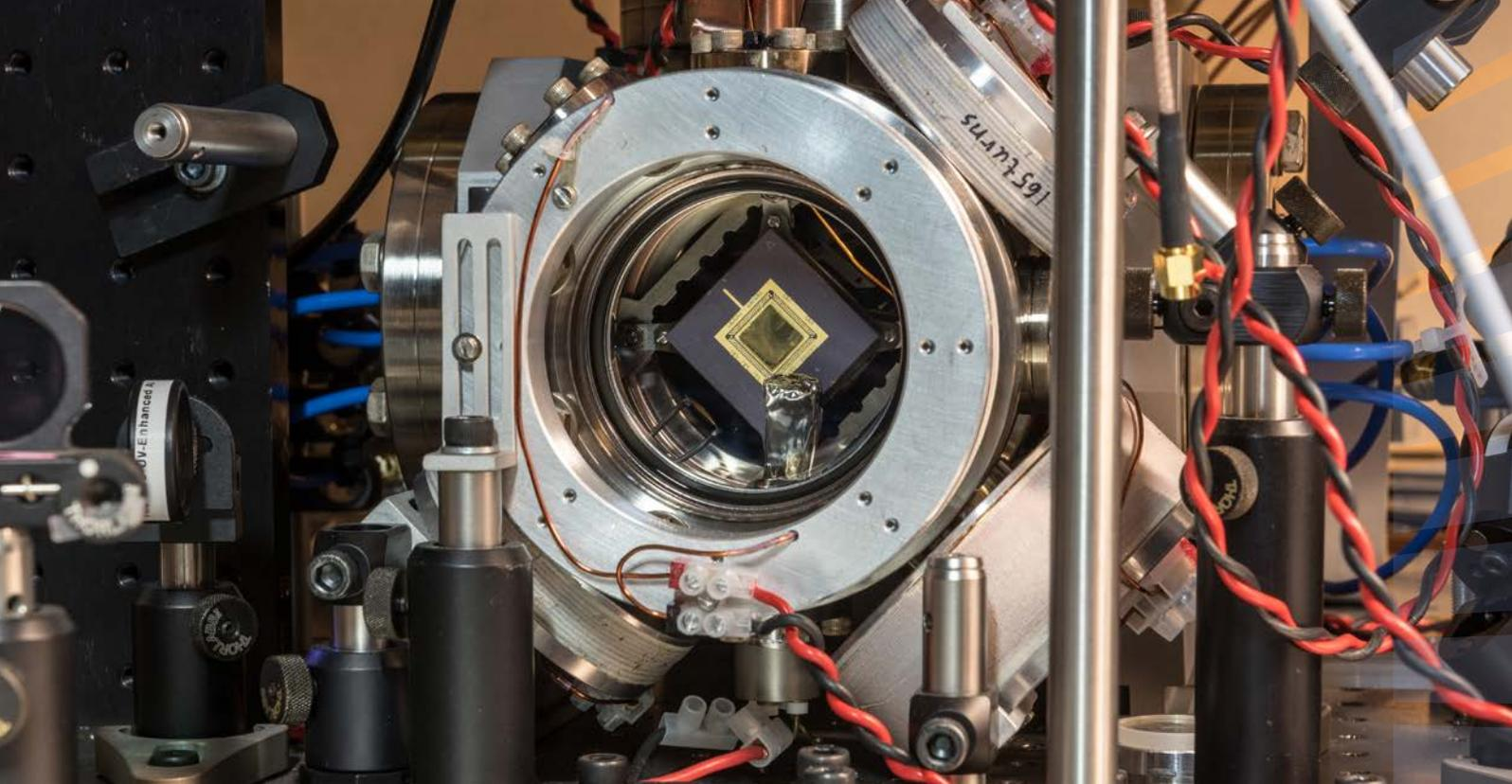
Ion trap on a microchip for quantum computing set inside a vacuum system in the Oxford Physics Lab / *Stuart Bebb*
