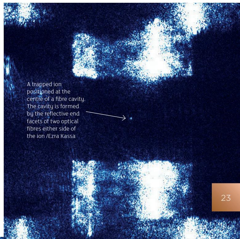
A trapped ion positioned at the centre of a fibre cavity. The cavity is formed by the reflective end facets of two optical fibres either side of the ion /Ezra Kassa
