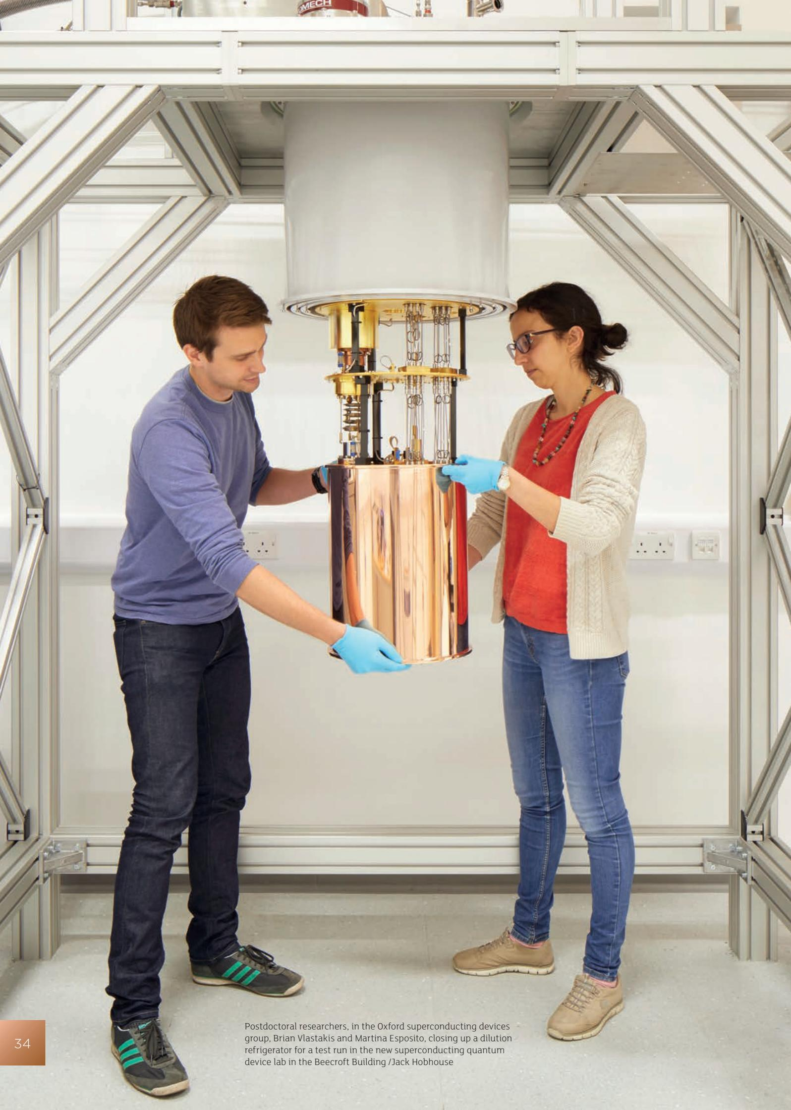
Postdoctoral researchers, in the Oxford superconducting devices group, Brian Vlastakis and Martina Esposito, closing up a dilution refrigerator for a test run in the new superconducting quantum device lab in the Beecroft Building /Jack Hobhouse
