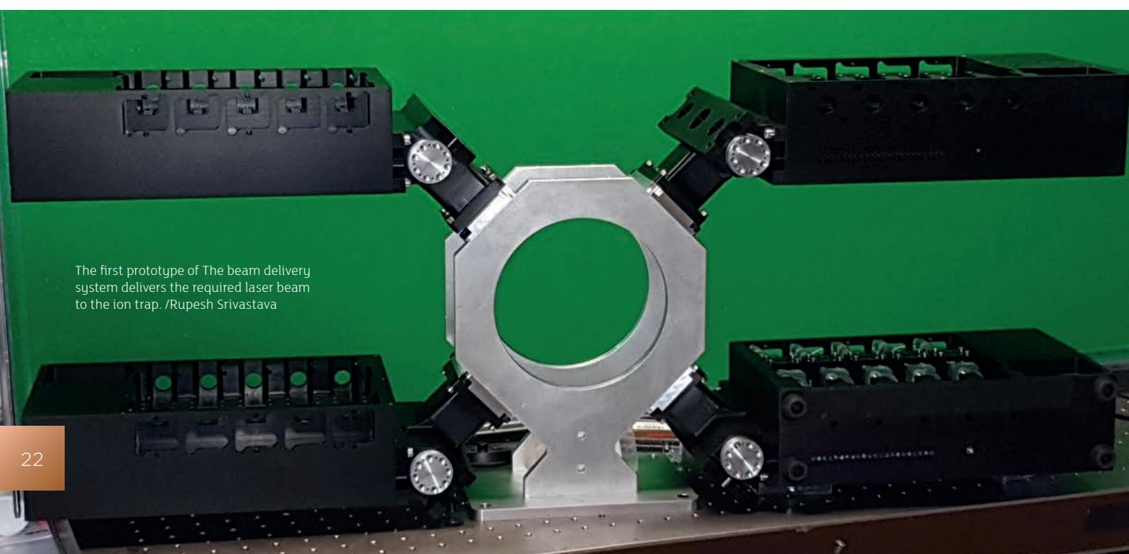
The first prototype of The beam delivery system delivers the required laser beam to the ion trap. /Rupesh Srivastava
