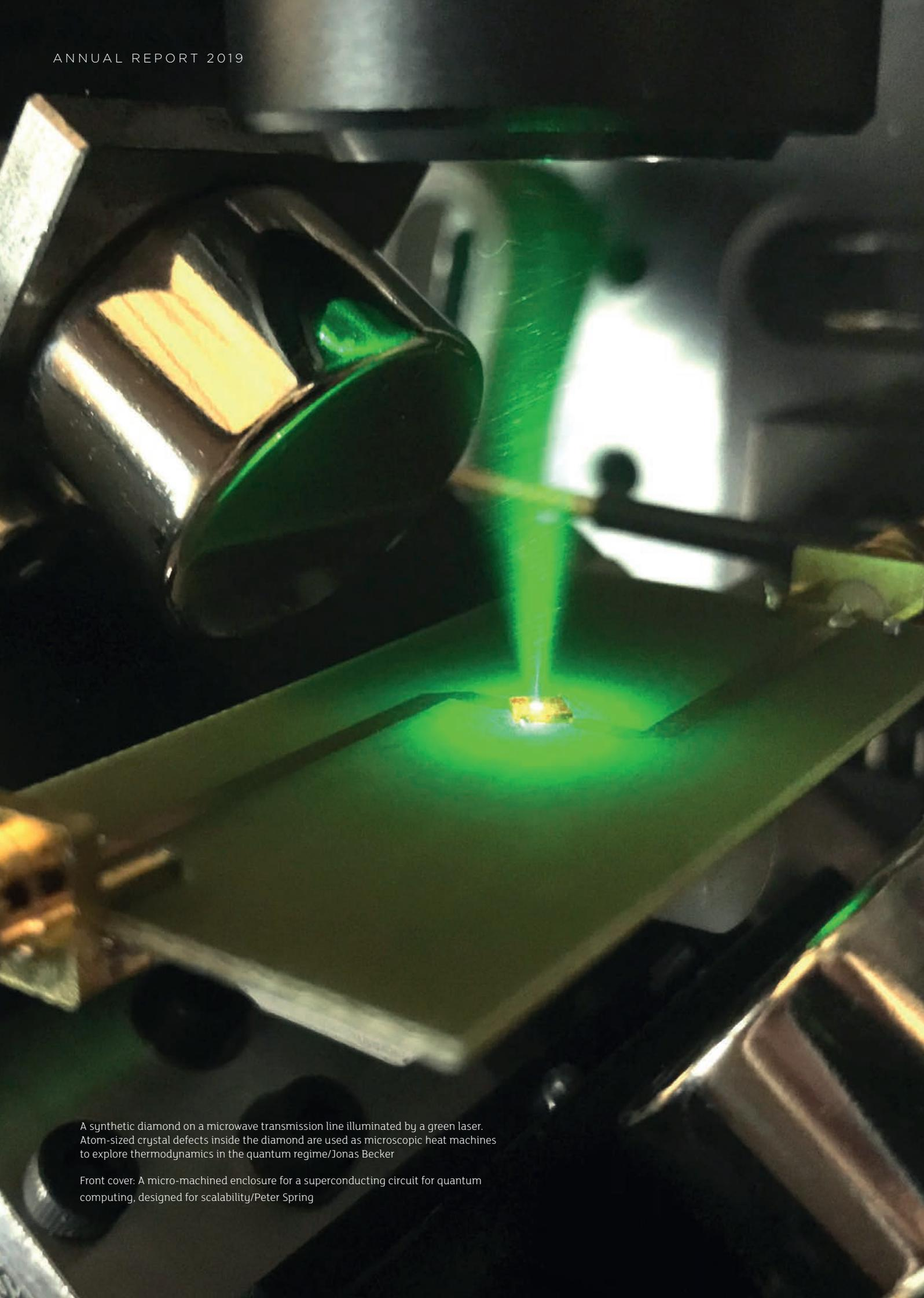
A synthetic diamond on a microwave transmission line illuminated by a green laser. Atom-sized crystal defects inside the diamond are used as microscopic heat machines to explore thermodynamics in the quantum regime/Jonas Becker
