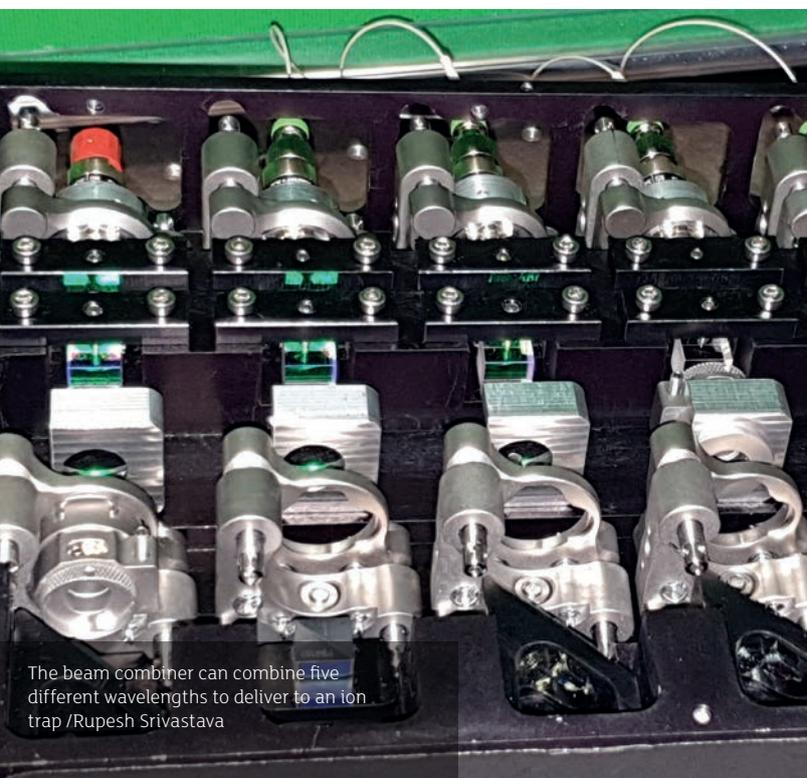
The beam combiner can combine five different wavelengths to deliver to an ion trap /Rupesh Srivastava
